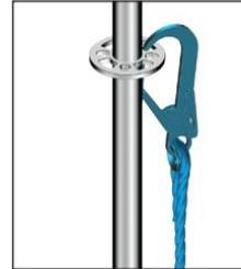
Attachment in the small or large hole of the rosette is possible.
