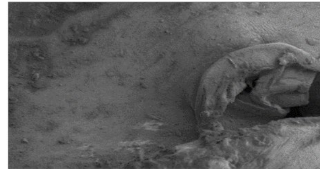
Figure 18. Day 40: A significant portion of the sheet is degraded, illustrating the culmination of the degradation process
