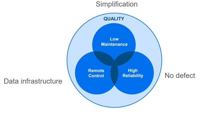
"Normally Unattended Installation" is a purpose-built facility which can be left unattended and still maintain its intended principal function through remote control from a distant location. (NORSOK STD S-001).
