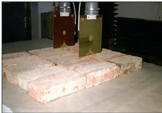
Fig. 8. Scanning of a brick wall structure by a pair of UWB antennas.
