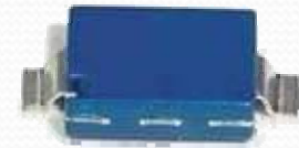
Integrated short range wireless transceiver size~20x20x2mm
