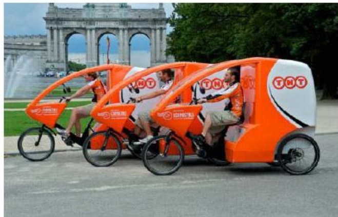
Third generation: 1,400 litres Capacity load: 180kg Speed: 20 km/h Length: 2.50m
