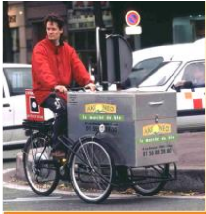
First generation: 400 litres Capacity load: 80 kg
