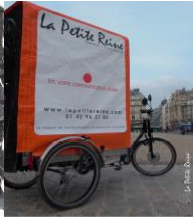
Third generation: 1,400 litres Capacity load: 180kg Speed: 20 km/h Length: 2.50m
