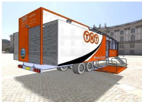
Trailer/truck fitted with typical depot facilities
