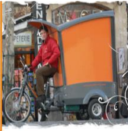
Second generation: 400 litres Capacity load: 150kg
