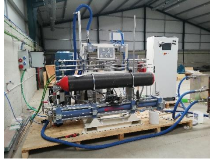
Compressor 50m 3 /h p_{in} : 10-40 bar p_{out} : 300-450 bar
