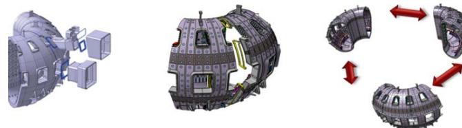
**VACUUM VESSEL.** Nine vacuum vessel sectors and 54 tokamak ports assembly . **ENSA**
