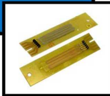
Silver & Copper Corrosion Sensors
