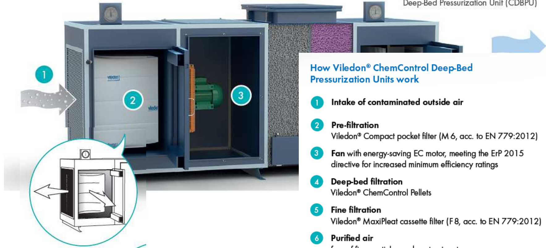
Figure: Example illustration of a complete Viledon® ChemControl Deep-Bed Pressurization Unit (CDBPU)
