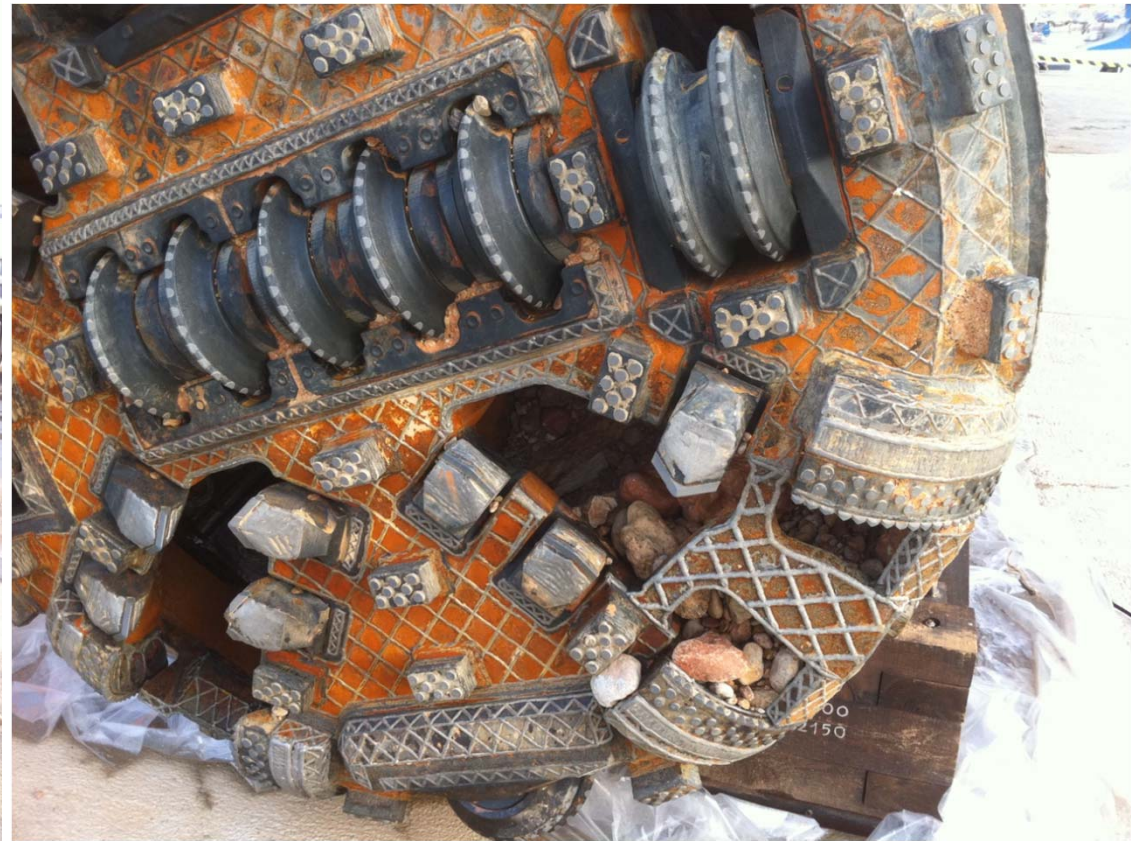
TBM – Detail of the cutting structure
